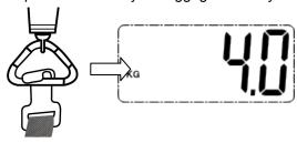
As soon as the weight is stabilized your scale will beep and the readout on the display will be locked.
