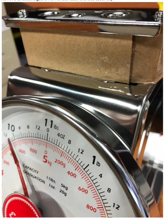
Use pliers to secure/grip the lock nut as pictured, and start loosening the screw with a Phillips screw driver from the load assembly.
