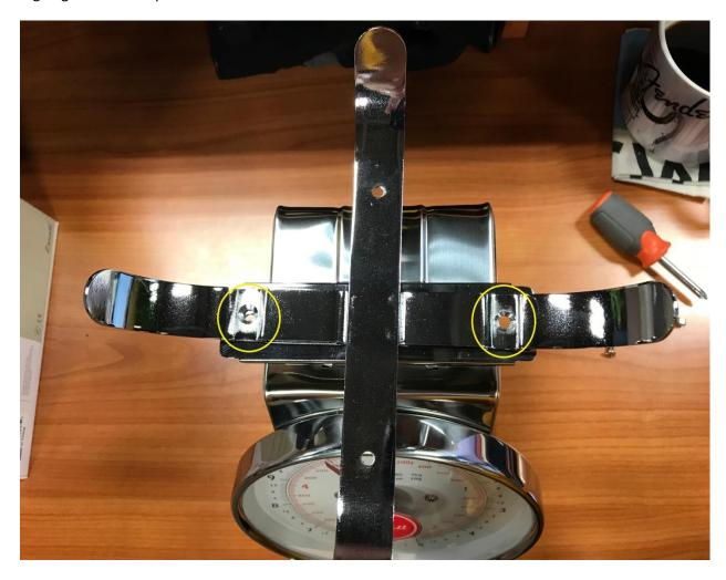
Place the screw into the aligned holes of the cross bracket and the load assembly.
