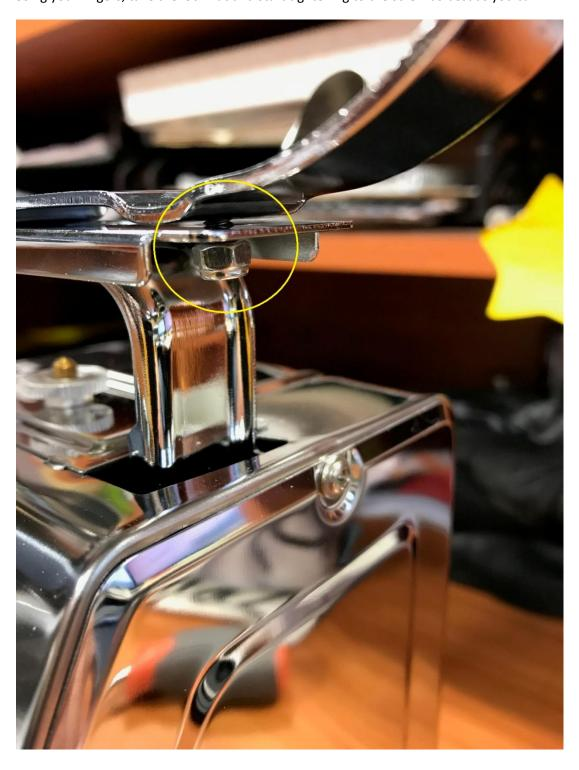
Finish off by using the pliers to hold the lock nut into place, and tightening the screw using the phillips screw driver as pictured.
