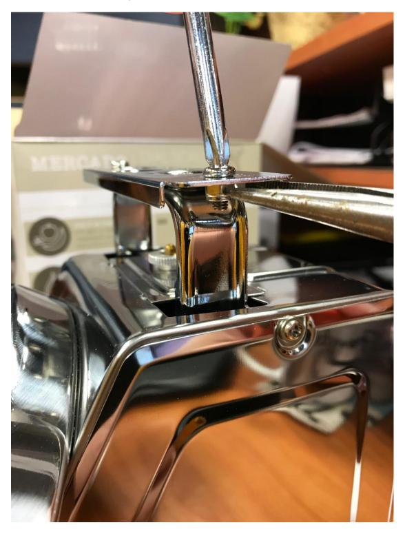
Once screws, and nuts are removed from both ends, place the cross bracket on top of the load assembly aligning the holes as pictured.
